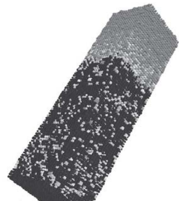
Figure 3: 3-D saturation profile simulated using the DYPOSIT model for a capillary rise problem.
