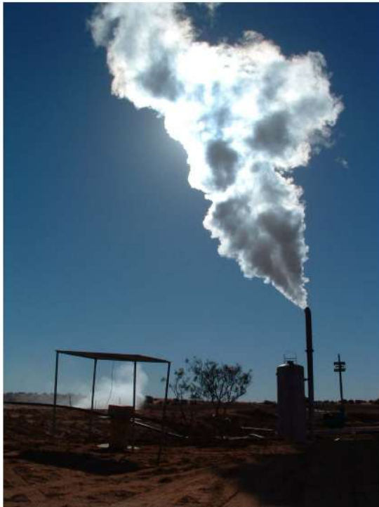
Habanero #2 well – Cooper Basin First HFR geothermal steam produced in Australia during clean-up flow test 23 April 2005
